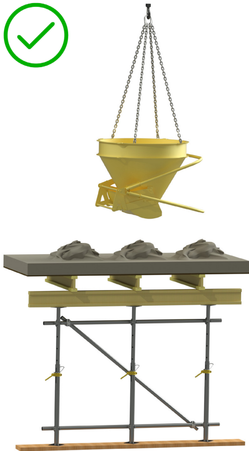
Apply uniform loads, to prevent prop buckling
