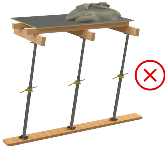
Falseworks may intend to turnover And or slide if it is subject to uneven loads
