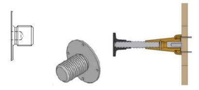
Note: Cone Positioner fixed to form face with 4 x Nails (30x80), subsequent removal with 14mm Allen Key.
